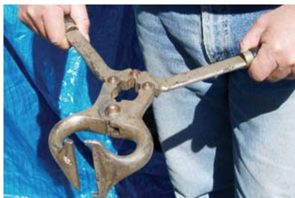
A Burdizzo® emasculator for non-surgical castration. (Hint – store your Burdizzo® with the jaws open to preserve spring tension.)
