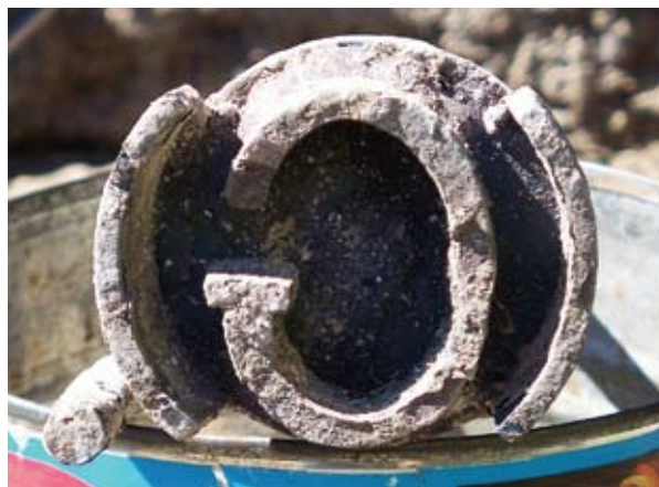
A symbol brand: the face of this one should be filed flat before being used.
